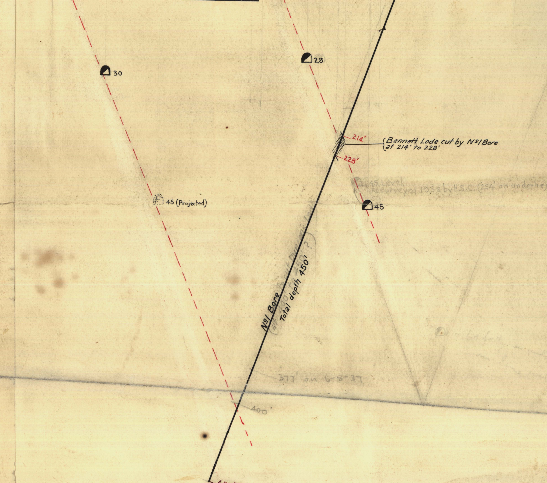
X Section thru' Bennett's & Duncan's Lodes at N°1 Bore.
